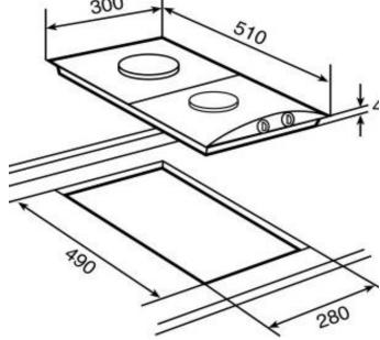
Cut hole must be with round corners in order to avoid cracking on the counter-top. **ATTENTION:**
